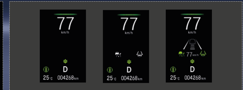
Adaptive Cruise Control Visual Display, CMBS & RDM Status, Digital Speed Display
