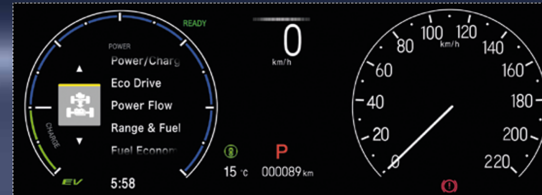
Large 17.7 cm (7 in) High Definition Full Colour TFT Meter with Multi Function Driver Information Interface
